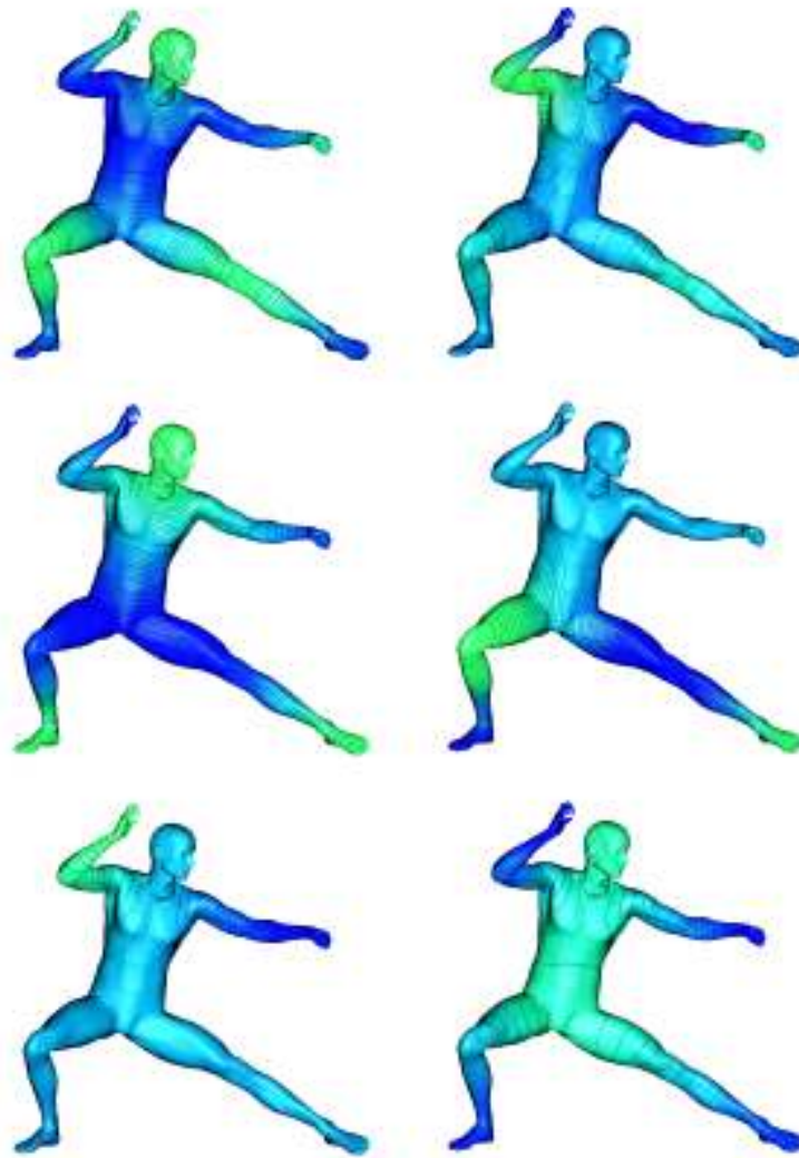
Figure 8.3. The first non-trivial eigenfunctions of the Laplace-Beltrami operator of a human shape. Colors and contours visualize the values of the eigenfunctions at each point of the shape.
